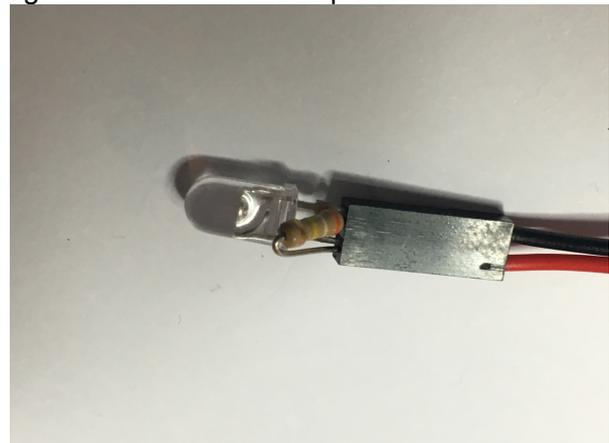
Slide both the phototransistor and resistor into the Dupoint connector.
