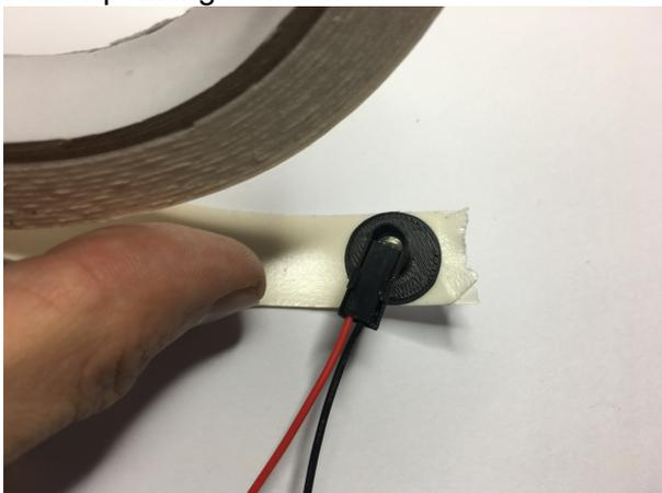
Cut out some double adhesive tape (the foam type works well) and stick it to the opening of the phototransistor holder.
