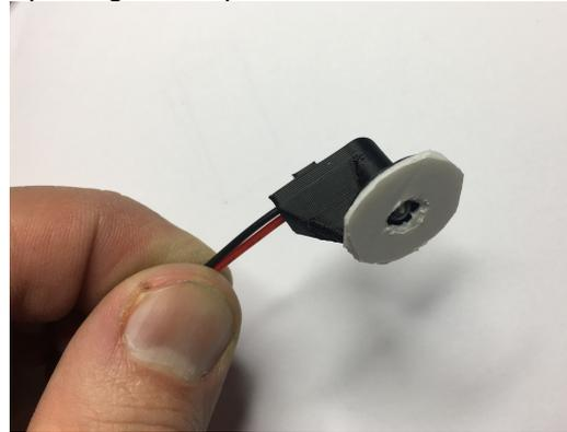
Make a hole for the phototransistor in the adhesive tape.
