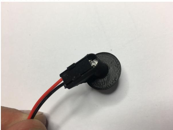
Bend the Dupont housing down into the positioning the picture. If you have the resistor as well it can be left outside the holder pointing forward.
