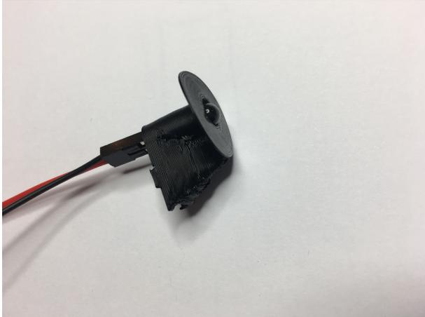
Push the phototransistor into the holder so that it sticks out 1-2mm.
