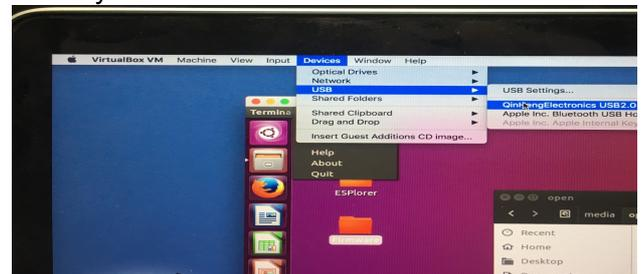
Once in the virtual machine in the menu click: Device -> USB and select Qin-Seng Electronics USB2.0-Serial (the name might vary on different operating systems). The name should appear after you plugged in the NodeMCU and disappear when you remove it.
