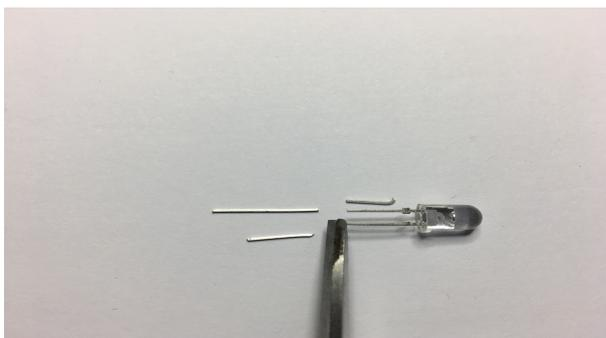
Begin with cutting the legs off from the phototransistor a bit.
