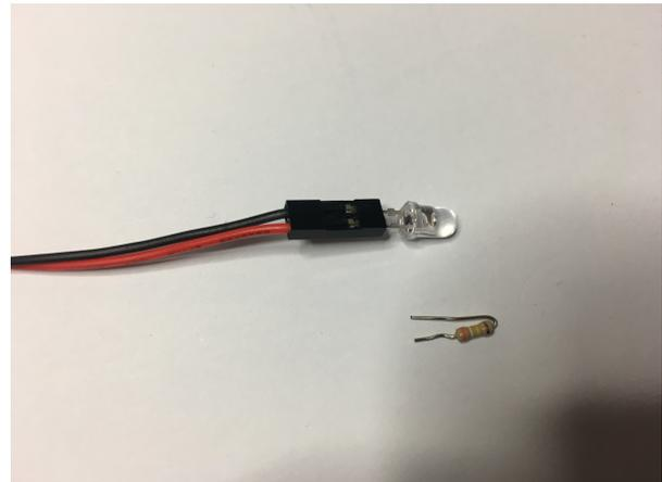
To increase the sensitivity of the phototransistor you might also have to add a resistor in parallel with it. In that case cut it as shown in the picture. The value of the resistor can be between 80-400kOhm. The smaller the resistance the more sensitive the phototransistor will be and the less light it needs to detect a pulse.
