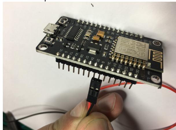
Connect a other side of the Dupoint cable to the GND and GPIO5 (situated next to
